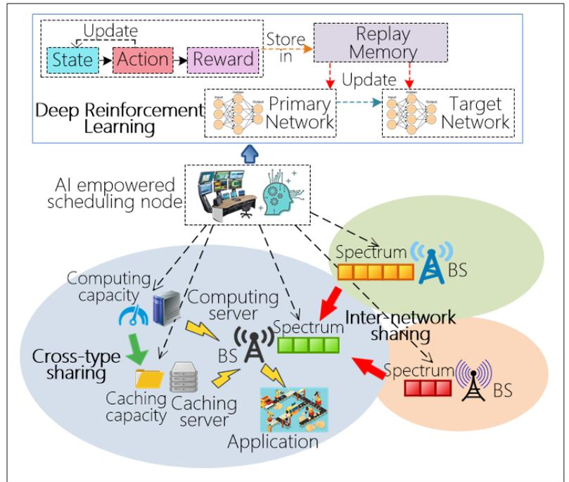
FIGURE 2. Cross-domain sharing empowered edge resource scheduling for 5G beyond IIoT networks.
