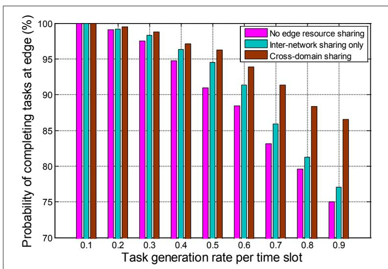
FIGURE 5. Probability of completing tasks at edge networks with different scheduling schemes.
